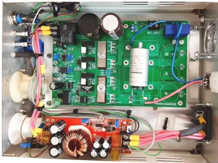
Fig. 3: The control section and the switching circuit of the proposed high voltage power supply.
