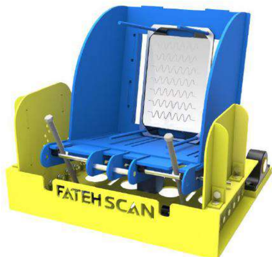
Figure 14. Representative test fixture for spatial resolution showing test object
