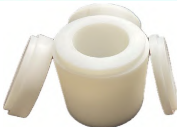
Figure 5. The polyethylene moderator made for the installation on the neutron generator.
