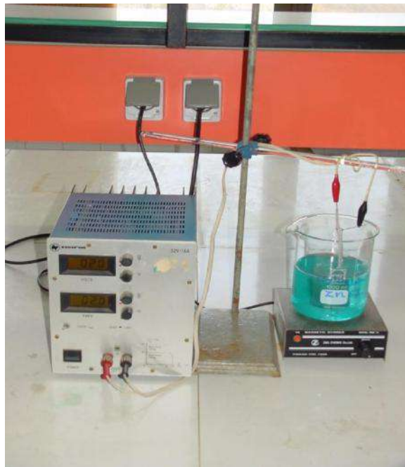
Figure 1. Electrolysis operation to remove copper impurity.
