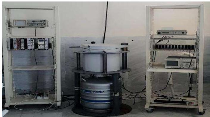
Fig. 1. The gamma spectrum system utilizes HPGe detector and equipment
