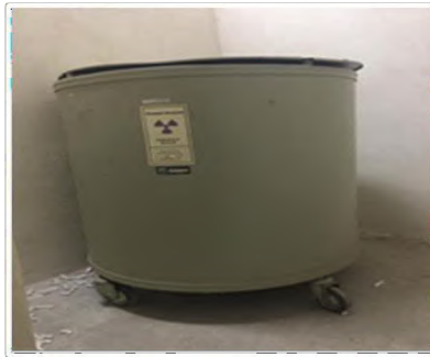
Fig. 1. Picture of source ^{226}\text{Ra} - ^9\text{Be} of Yazd University
