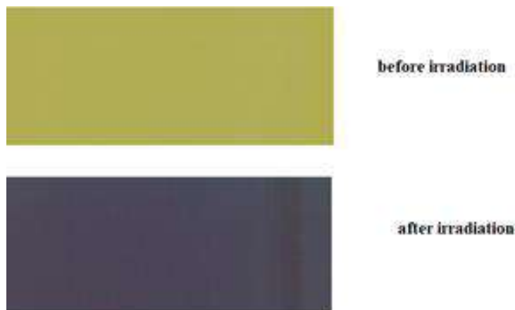
Fig. 4: The Gaf-chromic films before and after irradiation
