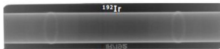
Fig.3. ^{192}\text{Ir} industrial radiography performance test
