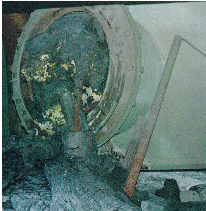
Fig.1 New formed uranyl phases (bright yellow aggregates) discovered on the surface of Chernobyl “lava” in steam-discharge corridor. Photo by scientists of Kurchatov Institute (1990).
