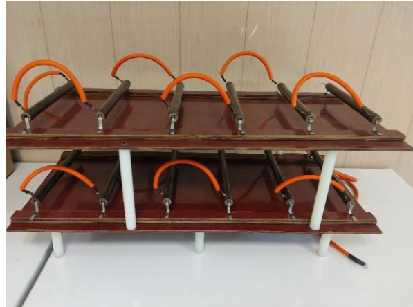
Fig. 3. Constructed magnetron equivalent resistance
