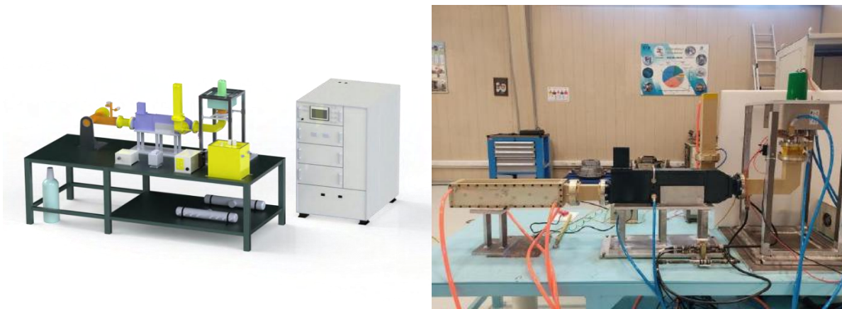
Fig. 1. Schematic view and picture of the completed radio frequency line.
