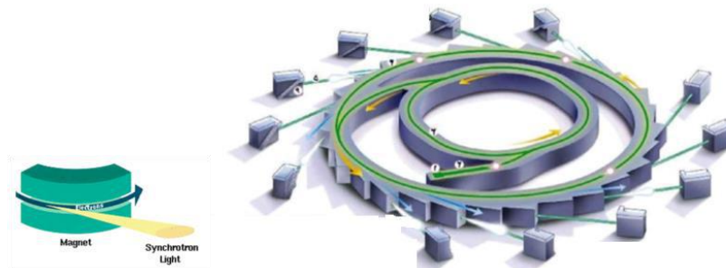
Figure 1: Schematic diagram of electron acceleration in synchrotron and how synchrotron radiation is emitted
