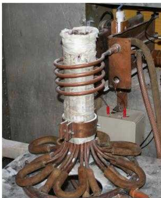
Fig. 3. The Induction furnace with the cold crucible developed in St. Petersburg University LETI(2).
