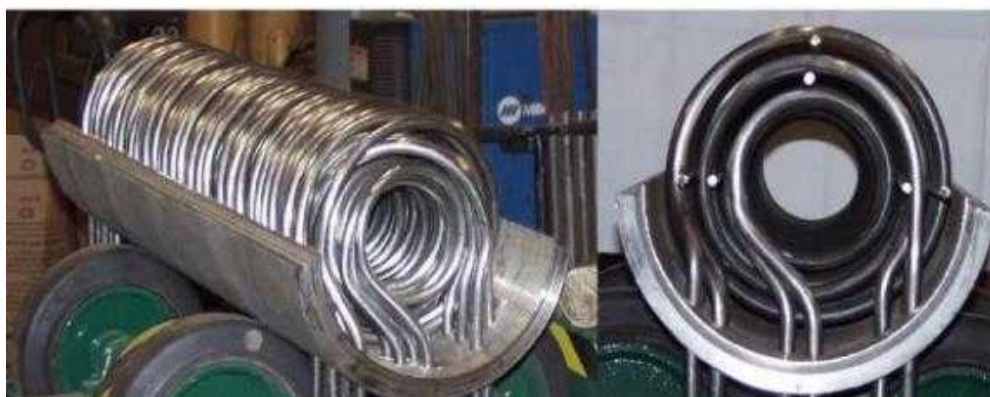
Fig. 2. Photographs of SG coil bundle arrangement [3]
