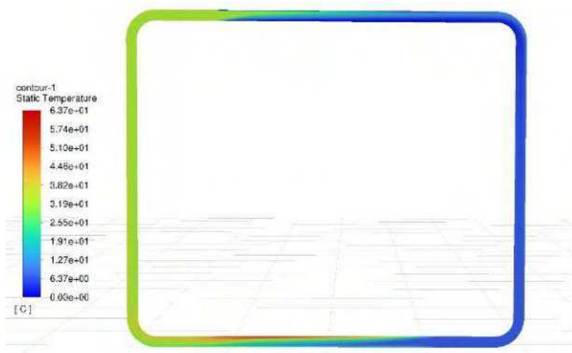
Fig.2 . Temperature distribution in the mini loop simulated using ANSYS Fluent
