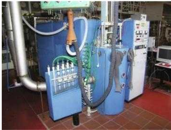
Fig. 4. Illustrations of the COMETA facility by (left) photograph and (right) schematic. 1: melting chamber; 2: supporting frame; 3: cold crucible; 4: inductor; 5: generator; 6: drive of frame (2); 7: ball and screw couple; 8: ventilator of the gas-purification system; 9: filter; 10: water cooling; 11: aerosol sampling; 12: pyrometer; 13: Digital Acquisition System(5).
