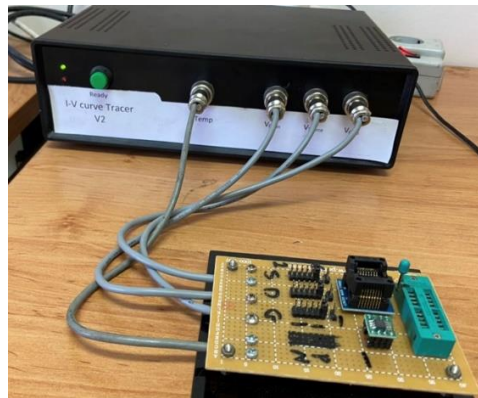
Fig. 2. The appearance of the current-voltage curve drawing device of MOSFET transistors made in Shahid Beheshti University [7]
