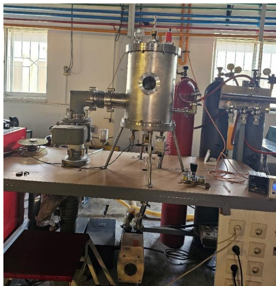
Fig. 1. Experimental setup of Direct-Current Diode Plasma (DC-DP)
