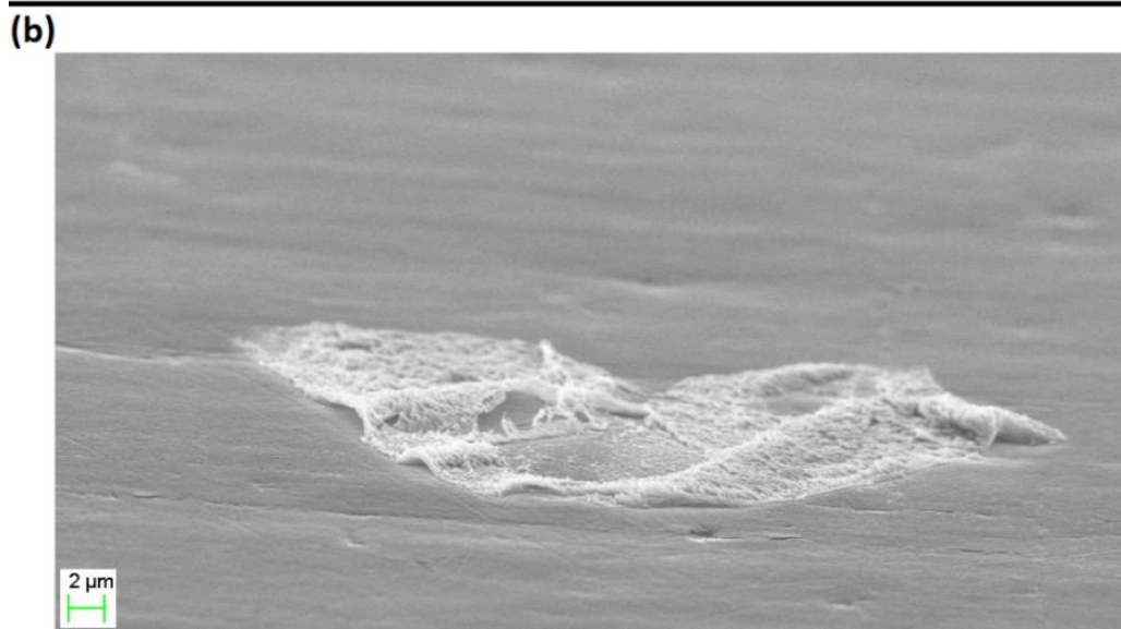
Fig. 2. (a) Coexistence of blisters alongside the nanostructures in W surface (b) absence of blisters in Mo samples
