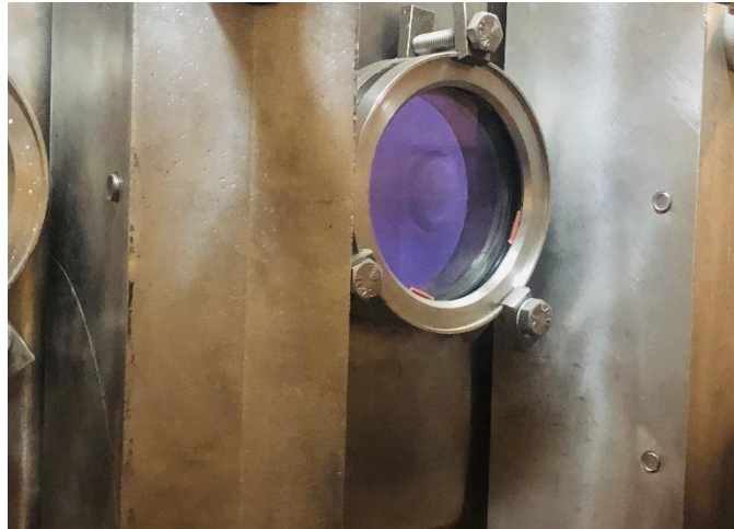
Figure 4: a view of glow discharge plasma formed in the Alborz tokamak
