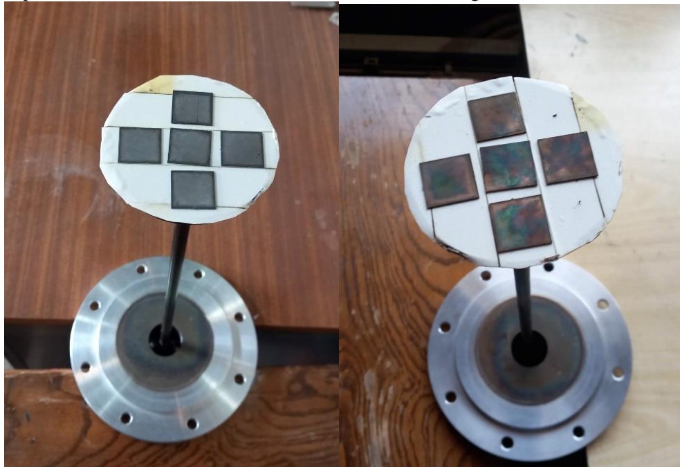
Figure 3. Five tungsten substrates were located on the feedthrough at 20cm distance from anode head. Left: before irradiation and right: after irradiation.
