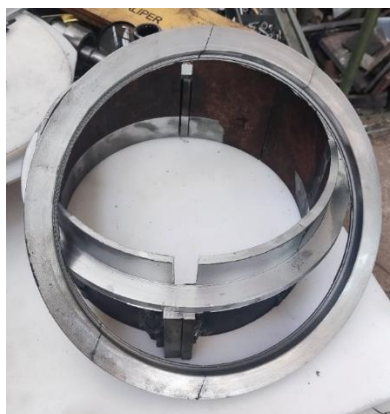
Fig. 5. Two chassis parts after machining. the clamping of both sides of the gear is also visible in the image.
