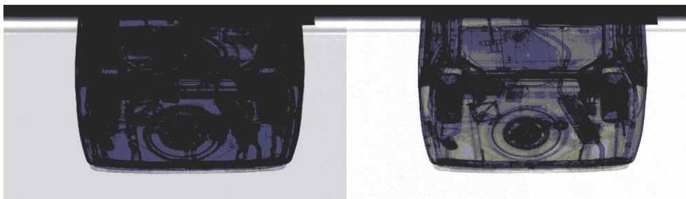
Fig. 4: High and Low images for a part of a car. The right side of the image is Low and the left side is High.
