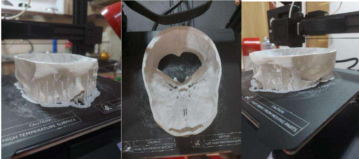
Fig. 5. Skull of AHD Prototype using FDM 3D printer
