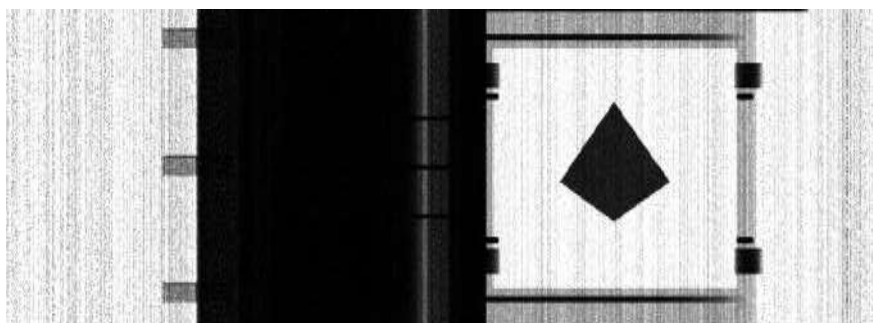
Fig. 5: X-ray image simulation with container and test object holder
