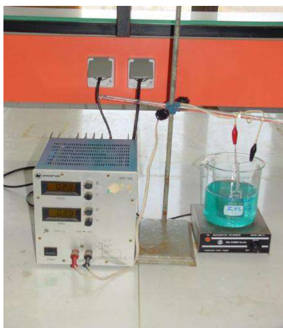
Figure 1. Electrolysis operation to remove copper impurity.
