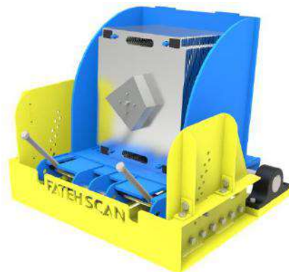
Figure 7. Representative test fixture for penetration and contrast sensitivity showing test object and steel plates
