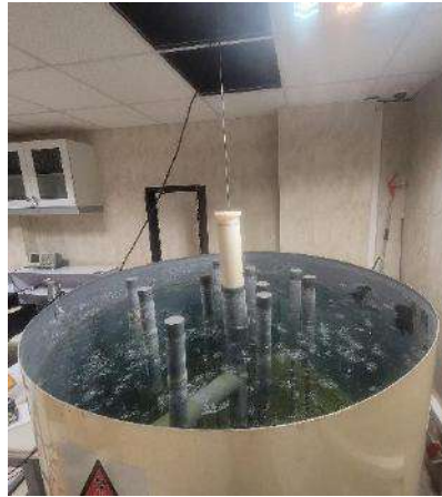
Fig. 3. Am-Be source is placed at the center of the iron tank containing water
