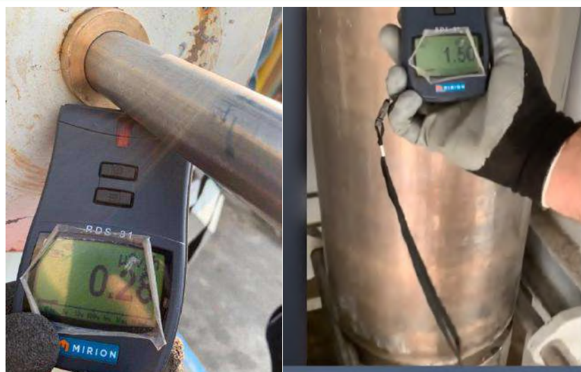
Fig. 3. Dosimetry of different regions of the gamma self- shielded system
