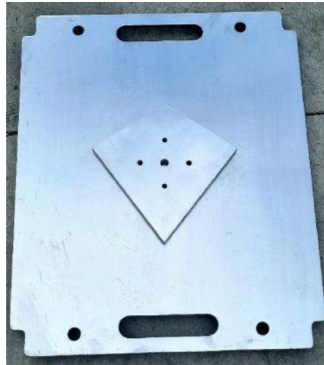
Figure 6. Make of penetration test object
