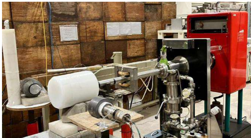
Figure 1. The 150 kV electrostatic accelerator that is used for the generation of neutrons via D-D reaction.
