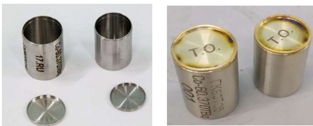
Fig. 1. Outer capsule (top) and inner capsule (bottom) of GC60T0 source model
