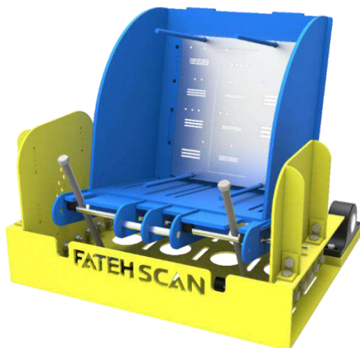
Figure 12. Representative test fixture for spatial resolution showing test object
