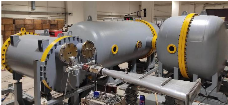
Fig. 3. a view of the Dynamitron accelerator built in NSTRI
