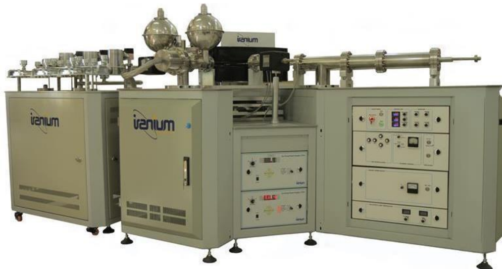
Fig.7. IRANIUM magnetic sector mass spectrometer with inlet system
