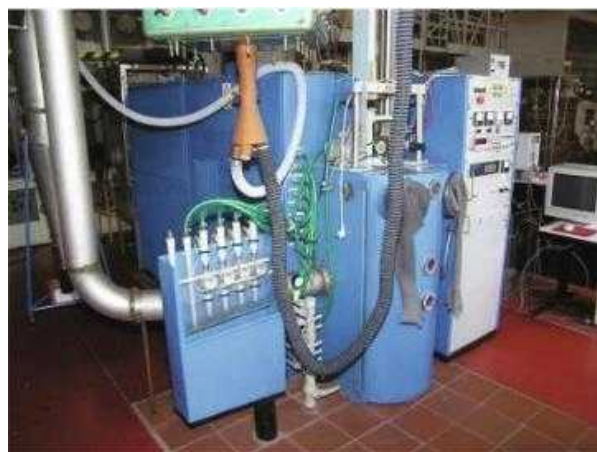
Fig. 4. Illustrations of the COMETA facility by (left) photograph and (right) schematic. 1: melting chamber; 2: supporting frame; 3: cold crucible; 4: inductor; 5: generator; 6: drive of frame (2); 7: ball and screw couple; 8: ventilator of the gas-purification system; 9: filter; 10: water cooling; 11: aerosol sampling; 12: pyrometer; 13: Digital Acquisition System(5).
