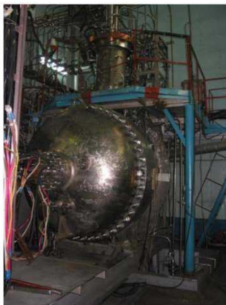
Fig.5. Physical form and layout of the Lava-B facility. 1: EMF (electric melting furnace), 2: crucible, 3: EMF inductor, 4: MR (melt receiver), 5: MR inductor, 6: concrete trap(13).
