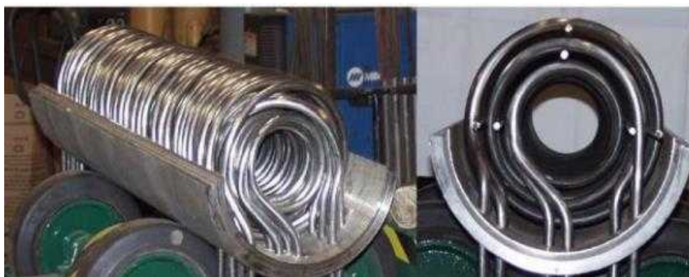
Fig. 2. Photographs of SG coil bundle arrangement [3]
