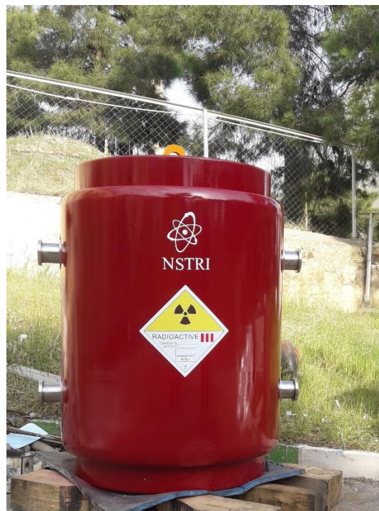
Figure 4: Constructed DPC at TRR [4]
