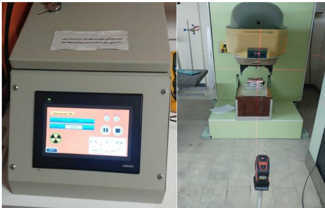
Fig. 3. Irradiation system of secondary standard dosimetry laboratory of Karaj and placement board of MOSFET parts.
