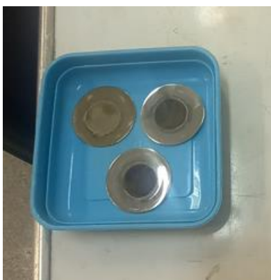
Fig. 6. Sources prepared using electrodeposition method
