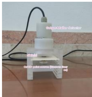
Fig. 2. Image of radiation protection experiment for pure ZnO and ZnO:Cu(10% and 20%)
