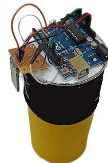
Fig. 2. The current-mode ionization chamber: Left: the detector sensor circuit. Right: the fabricated detector.
