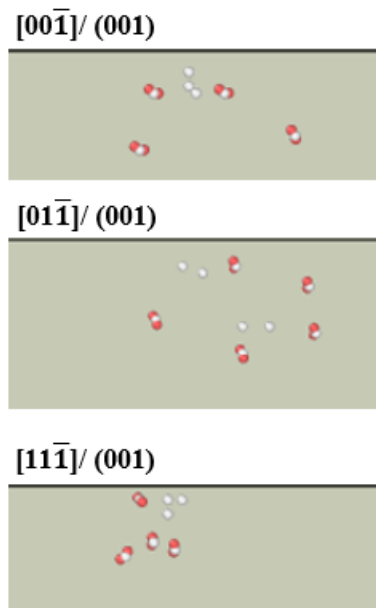
Fig. 4. The defect configuration diagram after the annihilation recombine of interstitials (red ball) and vacancies (white ball) in different directions.
