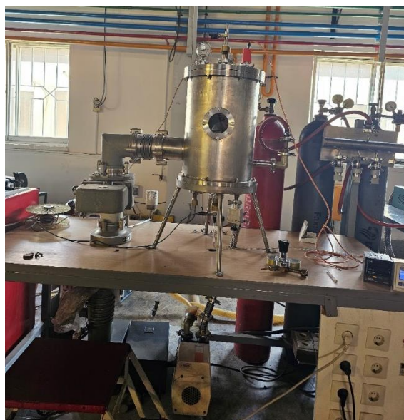
Fig. 1. Experimental setup of Direct-Current Diode Plasma (DC-DP)
