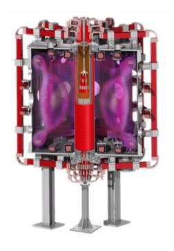
Figure 18: SMART cross section with negative triangularity plasma [7]
