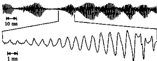
Fig. 7.1.1 Oscillations of the poloidal magnetic field measured outside the plasma (JET).
