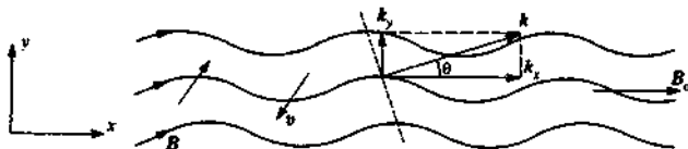
Fig. 2.24.3 The magnetosonic wave has velocity oscillations in the plane containing B_0 and k
