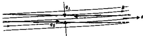
Fig. 7.16.1 The MARFE region, shown shaded, is cooled by radiation and heated by the stabilizing perpendicular and parallel heat fluxes.
